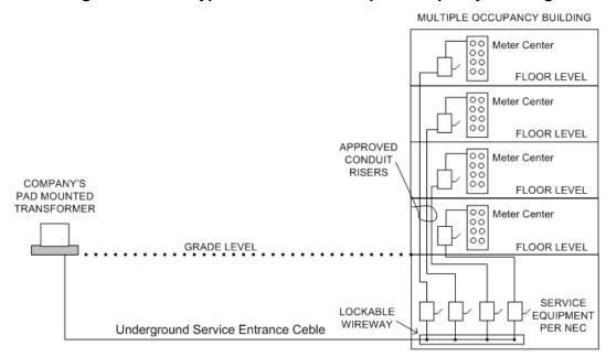
Figure 4.4.7.3-1 Typical Service to Multiple Occupancy Building
