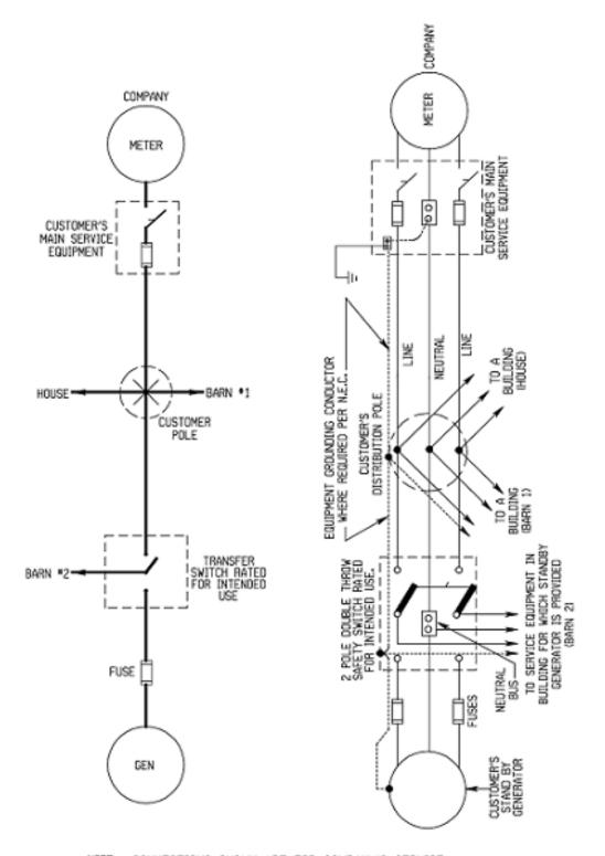
NOTE: CONNECTIONS SHOWN ARE FOR COMPANY'S SERVICE BEING SINGLE PHASE 3 WIRE 120/240 VOLTS.
